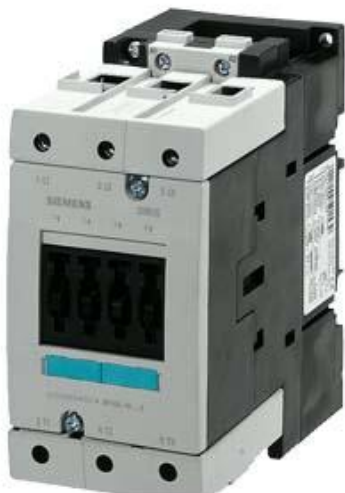
CONTACTOR, AC-3 30 KW/400 V, AC 220V 50HZ/240V 60HZ 3-POLE, SIZE S3, SCREW CONNECTION
